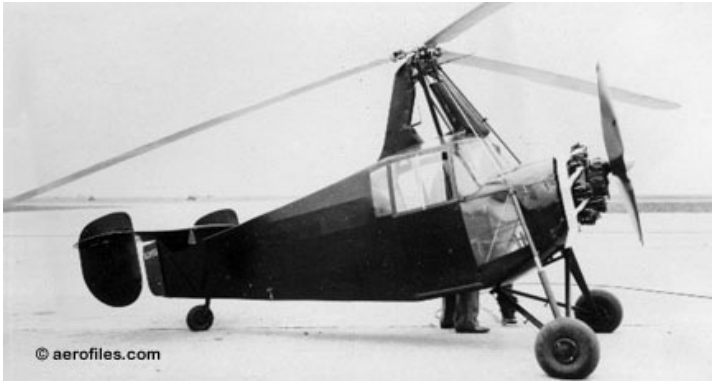
PA-22 1932 84hp Pobjoy Cararact Experimental wingless with a three-blade, foldable rotor system. Side-by-side cabin; width: 7'10". First road able autogyro built→
